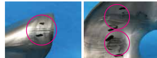
Product molded with unprocessed dies. 未処理金形成型品
