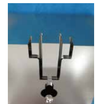
Stationary insert: After OX-FSP+OX-Polish process. 固定入子:OX-FSP+OX-Polish処理後
